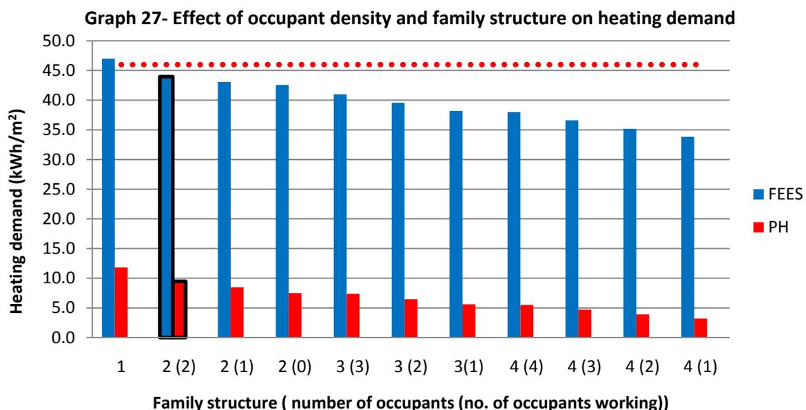
Table 48- Heating load for different family structure
