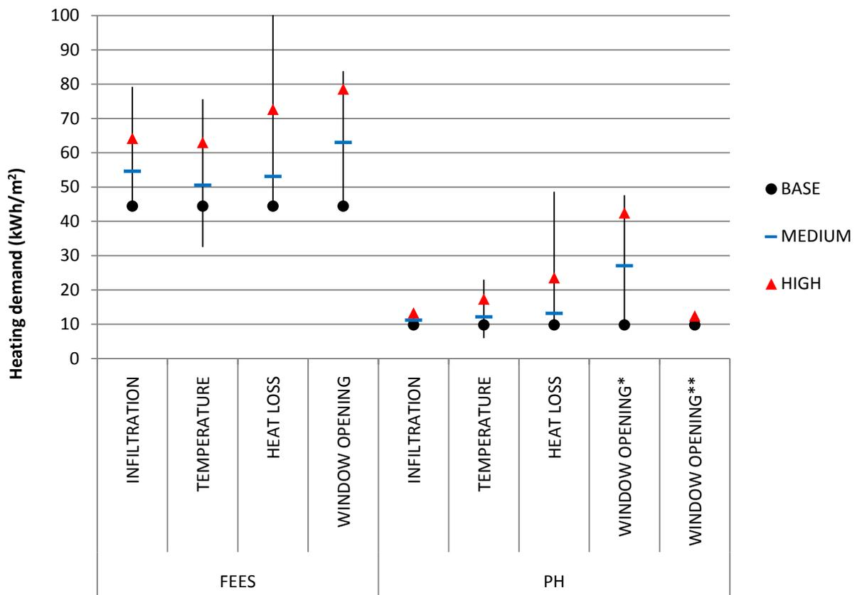
\*Effect of window opening behaviour in case MVHR was not used- not realistic for Passivhaus standard
