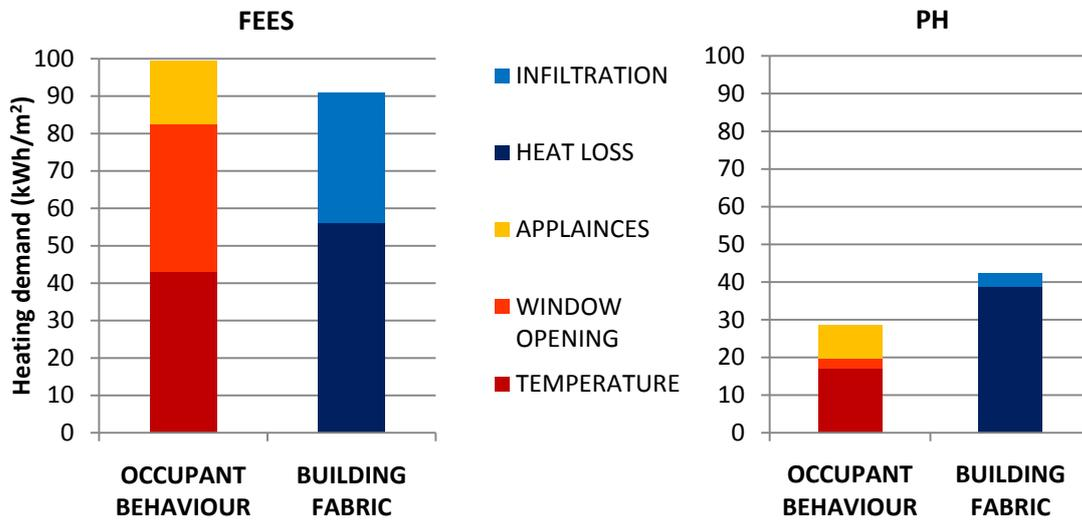
**Graph 22- Comparison of estimated maximal realistic variations in heating demand due to occupant behaviour and deterioration of building fabric for FEES and PH house**
