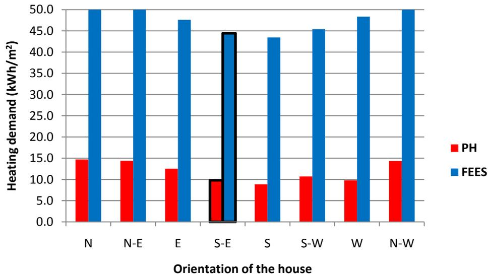
This indicates that site constrains in terms of building orientation can have much more significant implications on heating demand and that that thus significantly higher quality of building fabric is needed if compliance is to be achieved regardless of these realistic constrains.
