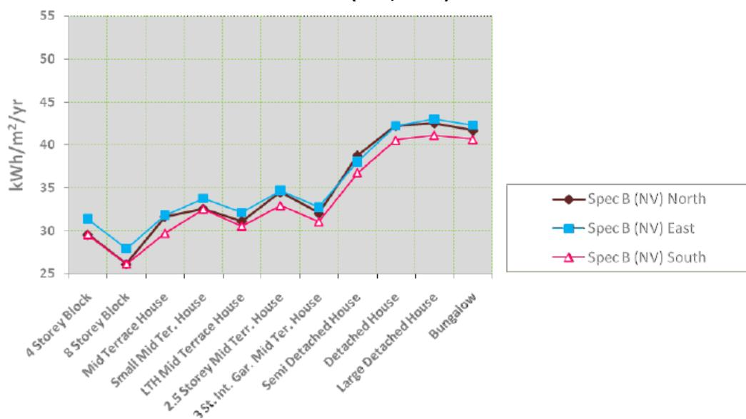
Considering that site constrains can be restricting in terms of use of optimal orientation, the model of the house is rotated in order to estimate maximal variations in heating demand. Variations in cooling load are not within the scope of this study but they are expected to be minimal compared to heating due to use of shading.
