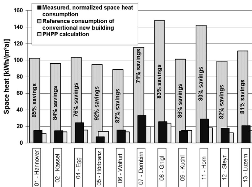
Graph 7- Space heat consumption normalized to 20 °C compared to the consumption of conventional new buildings and to the values calculated by PHPP (Schnieders, 2003, p. 346)
