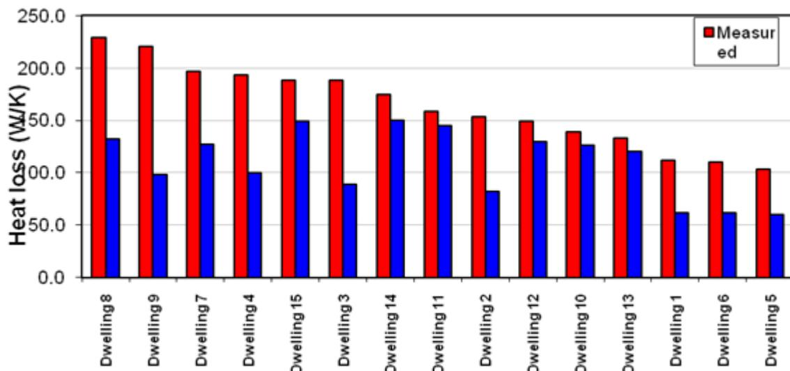
Figure 5- Measured and predicted whole house heat loss in 16 new low energy dwelling (Wingfield, et al., 2009, cited in GHA, in press, p. 25)
