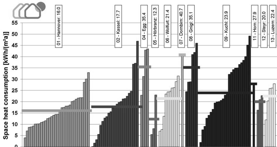
Graph 6- Measured space heat consumption of CEPHEUS buildings (for every project mean is displayed as a horizontal bar) (Schnieders, 2003, p. 345)
