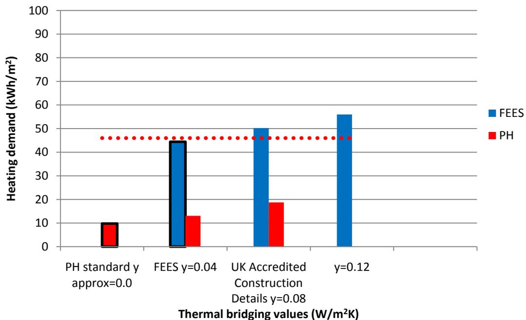
On the other hand, if in the PH house, thermal bridging goes up to 0.04 W/m<sup>2</sup>K Passivhaus compliance would still not be compromised (Table 35).
