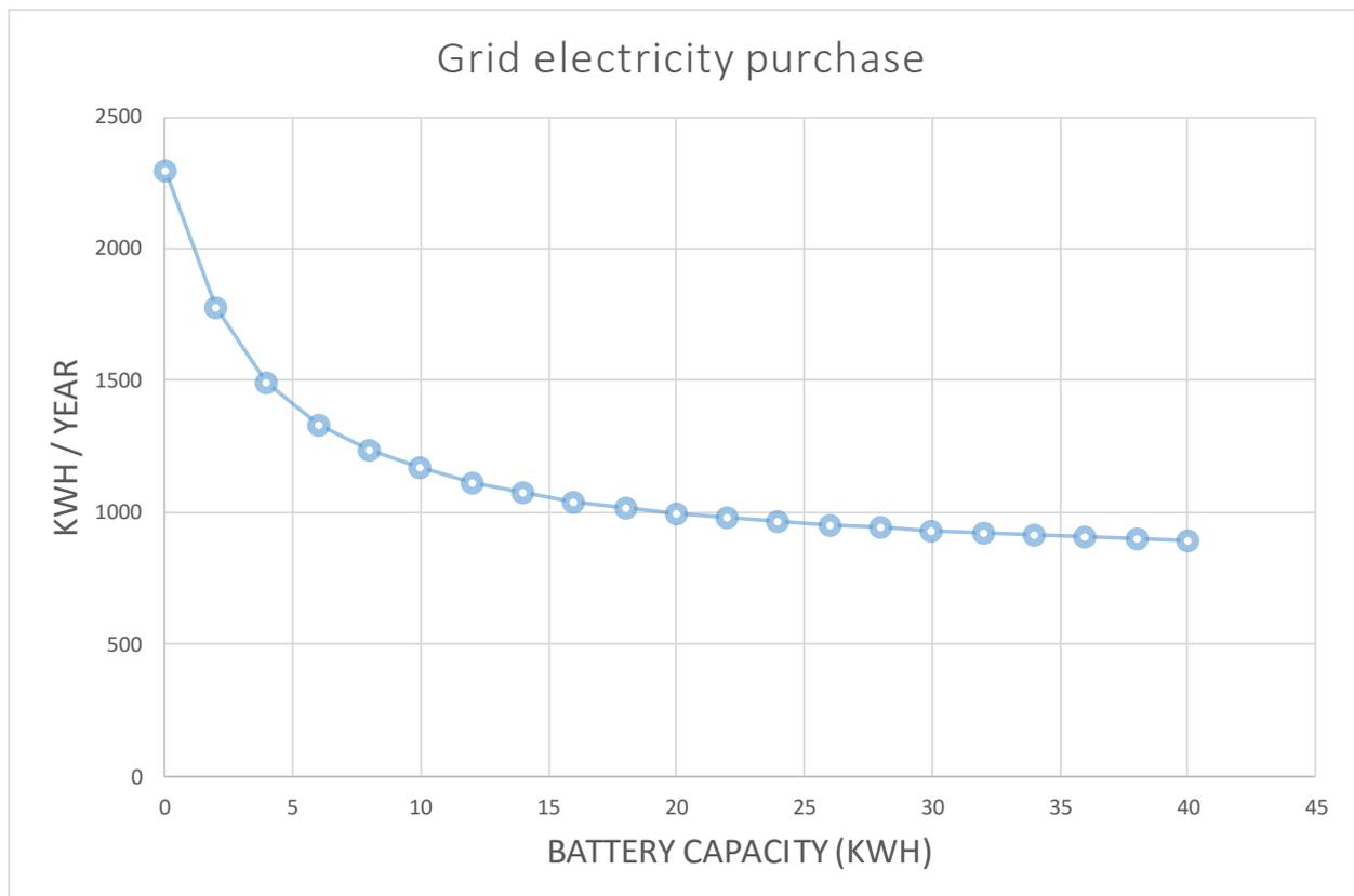
For this indicator, we can also notice a logarithmic behavior: the first kWhs installed allow a reduction of grid electricity purchase. However, the reduction is limited. This behavior is due to the winter period.
