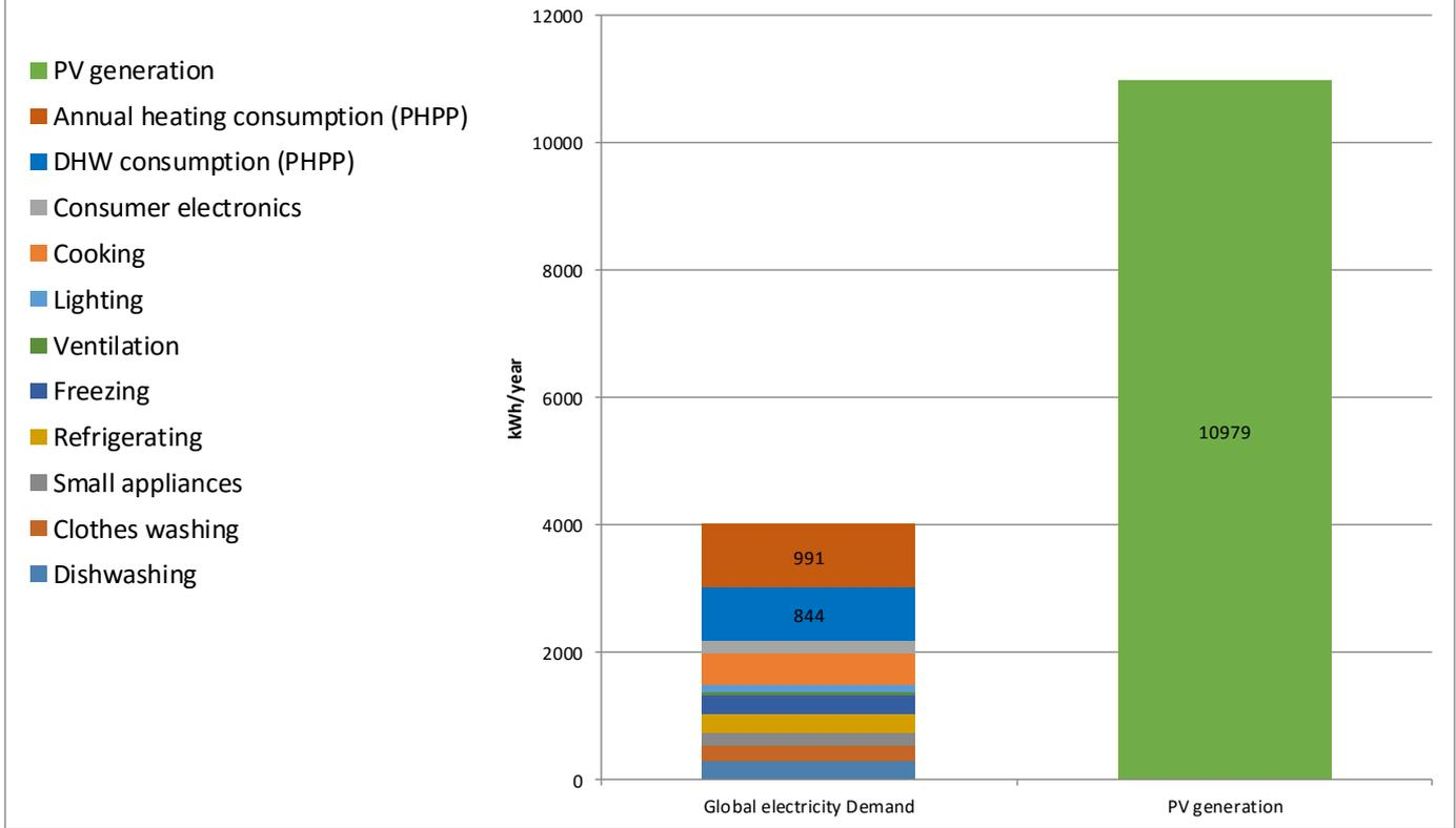
On an annual basis, we can notice that the PV production is about 2.5 times higher than electricity demand.
